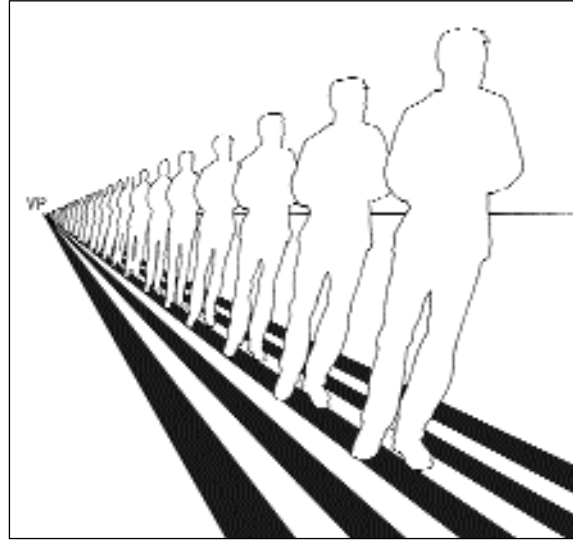
The figures in this long lineup appear smaller the closer they are to the vanishing point.
